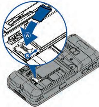
Figure 18. Insert an Optional MicroSD Card
