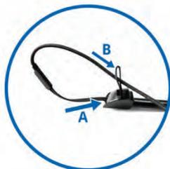
Figure 16. Insert the Strap into the Stylus
