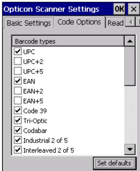
From the code options tab barcode types that need to be supported can be enabled or disabled. Some of these barcode support some standard options that can be reached by tap and holding a specific barcode type. When this is done popup menu appears and click the code option. Now the code option menu is shown.
