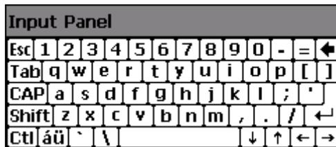
The input panel or also called virtual keyboard can be used to input data. The input panel will not come up automatically when the cursor is placed into an edit field. The keyboard can be controlled from the taskbar. If the automatic mode of the input panel is wanted a registry key needs to be changed.
