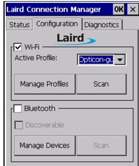
The Configuration tab allows Wi-Fi and Bluetooth to be enabled and disabled. It also allows users to manage Wi-Fi profiles, Bluetooth devices, and to scan for both.
