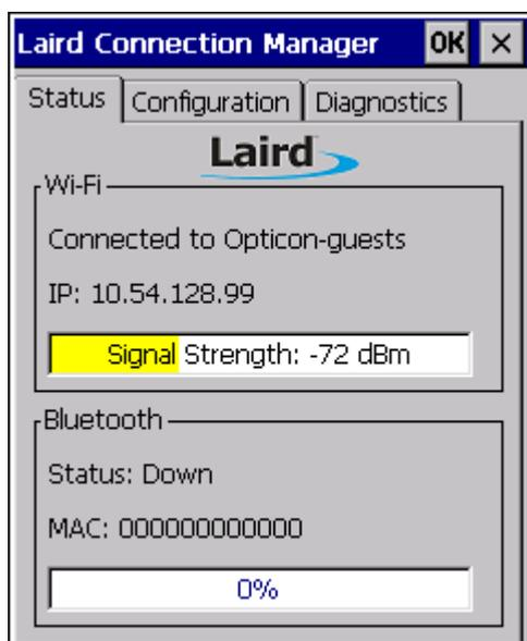
The status tab is divided into Wi-Fi and Bluetooth sections. The Wi-Fi section provides status information on the radio's Wi-Fi connection between the client device and the access point to which it's associated. The Bluetooth section provides status information on the radio's Bluetooth connection between the client device and the destination device.
