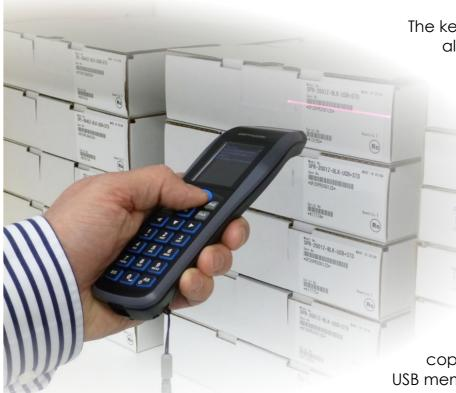
The keypad on the barcode scanner allows you to enter a code if the barcode is damaged and / or add an amount to the last barcode scanned.
